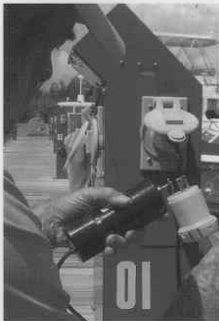
Marinas can use a newly developed technique, Mk-3 Bonding Test, to determine the integrity of the deck and boat-bonding system.
